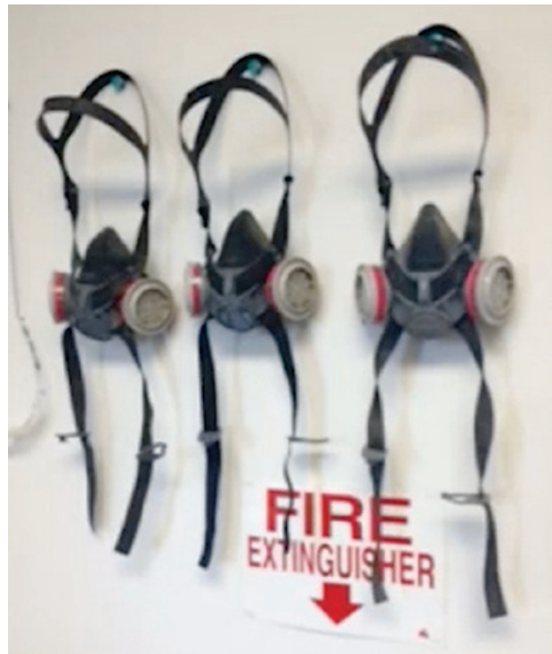
Respirators improperly stored: hanging in the open.
