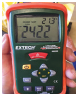
When a second 90 degree bend appears in the duct, air flow decreases 483 CFM or approximately 16.6%.
