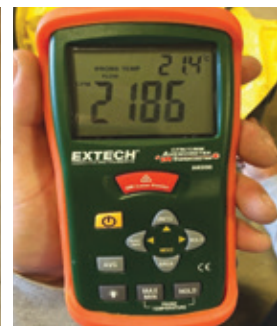
When we install a filter, air flow decreases 719 CFM or 24.75%.
