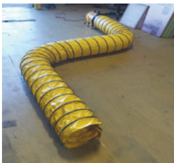
When a second 90 degree bend appears in the duct, air flow decreases 483 CFM or approximately 16.6%.
