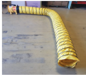
When the duct encounters a 90 degree bend, the air flow decreases 271 CFM or approximately 9.3%.
