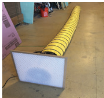
When we install a filter, air flow decreases 719 CFM or 24.75%.
