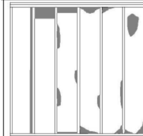
No more than 10% of surface area of insulation compressed or incomplete fill, by up to 30% (70% or more of intended thickness) is acceptable for "Grade II".
